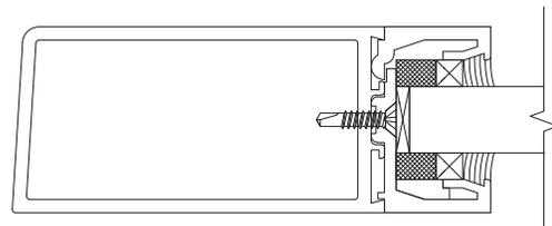
Note: Details show open for 9/16" large missile impact glazing. Option for 1" large impact missile glazing also available.
